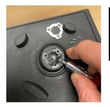
Hold the motor drive (20) in position with multiple slip joint pliers, and unscrew the fixing screw (19) using a TORX wrench (anticlockwise)
