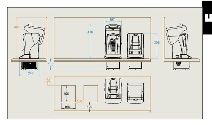
Make sure there is sufficient clearance (behind, above, below) for proper installation and operation of the appliance.
